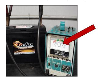
**Note:** Cranking a starter motor with the battery in a low voltage condition, can cause the starter's solenoid contacts to weld together, resulting in an over-cranking situation, burning out the starter motor.
