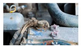
**4.** Ensure all terminal connections to the battery posts are secure & tight.
