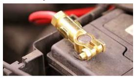
5. The battery should be fully charged, with the vehicle's engine off. Terminal voltage OCV (Open Circuit Voltage) for maintenance free batteries must read 12.6 volts at 100% charge. A minimum 12.4 volts at 75% charge is necessary to properly test the vehicles electrical system. Terminal voltage OCV of new batteries must register 12.5 volts before installation. Recharge & re-test any battery that does not meet these required voltage readings.
